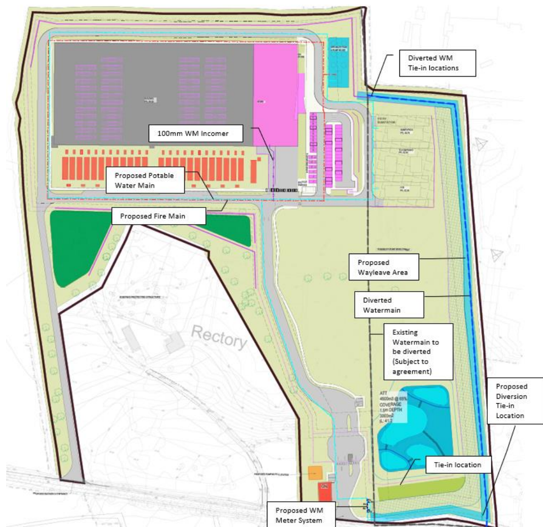
Figure 14.5 Proposed Watermain Diversion with Tie-in locations (Source: CSEA)
